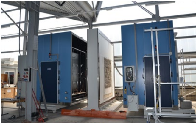
Figure 19: Stonewall mock-up in INTENT hot box
