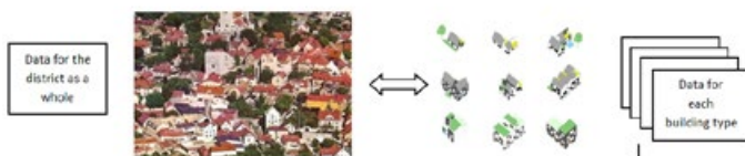
Figure 39: Building stock categorisation: from whole district data to data for representative sample buildings
