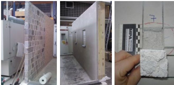
Figure 21: EOTA wall for durability test under harsh weathering conditions – before (stone masonry, left) and after plastering (timber frame, middle) as well as pull-off-test (right).
