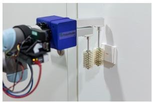
By using its flexible cleaning tool, DeKonBot 2 can disinfect different objects by wiping, in addition to door handles and knobs also elevator buttons or
