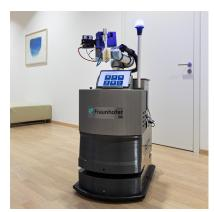
For regular operation, the tablet is attached to the robot which navigates autonomously from one object to be cleaned to the next.
