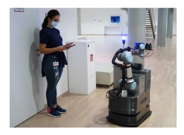
During the practical tests, members of the cleaning staff could program the robot using a tablet.
